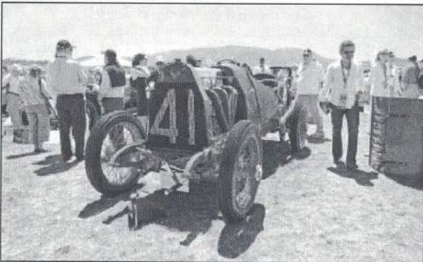
Pebble Beach had a unique class, the "10+ Club". In the early days, the way to more horsepower was more displacement. This 4-cylinder Fiat S74 from Oregon boasted a 14 liter engine [not 1.4: pistons like buckets?], and won the class.
