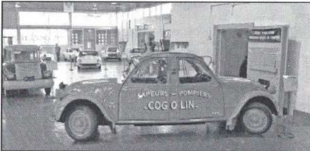
A replica of the 2-headed '52 Citroen 2CV which served the Cogolin, France fire & rescue service: 2 independent fronts welded together so they could get down a blocked mountain road.
