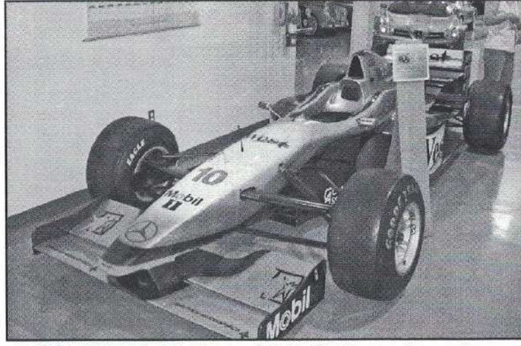
A 1997 McLaren-Mercedes MP 4-12 F1 car, driven by David Coulthard to a win in Japan; 3.0L V-10, 16,000+rpm weighing 600 kg including the driver.
