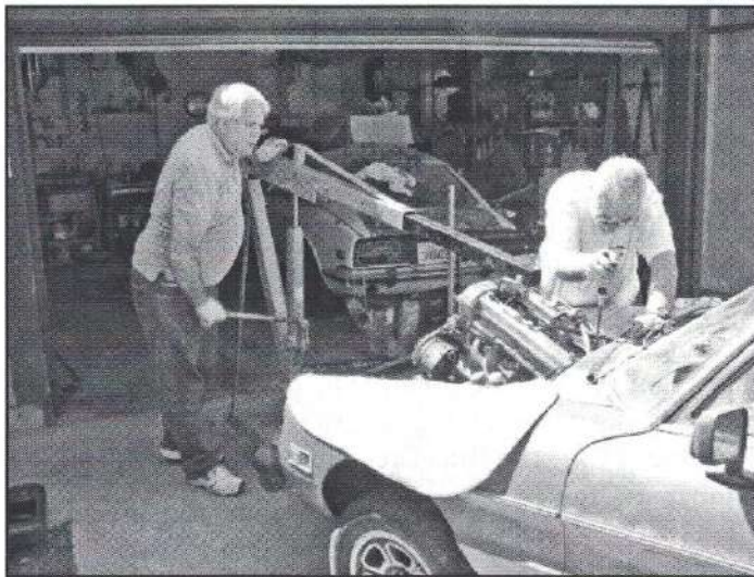
Gene starts to hoist the engine out while Norm looks for interferences.
