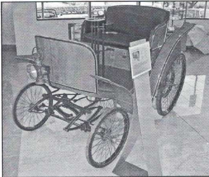
An 1895 Benz Velo, the highly successful first production car, with over 2000 delivered. It has 2.75 hp @ 600 rpm, for a top speed of 15 mph.
