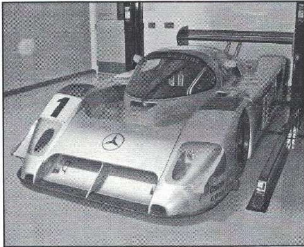
The 1991 C291 Group C Racer, with a 3.5L V-12, 650 hp @ 13,000 rpm, max speed of 239 mph, 1800 lbs; driven by J Mass & JL Schlessler.
