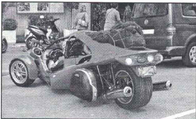
A T-Rex 3-wheeled motorcycle, Honda powered. It leans mechanically in turns, and looks well equipped for travel in Europe.
