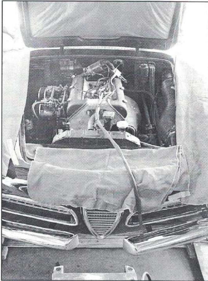
Under the hood -- the 2000 Spider engine is a bit different than the late 2.0 liter, and has a cast iron block. Notice the individual cam covers are mounted on a slanted face rather than horizontal like Doug Bender's engine to the right. This was a transition design between the cast-iron 1900 series and the aluminum Giulietta, which has more power with 1300 cc..
