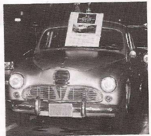
The Bergantin. Note the shape of the Alfa grille opening behind the lower grille.
