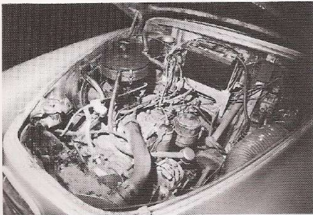
The Kaiser flathead six-cylinder of the Bergantin
