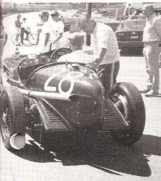
1929 Miller 91 Front-Drive—Note Frank Lockhart's original intercooler design
